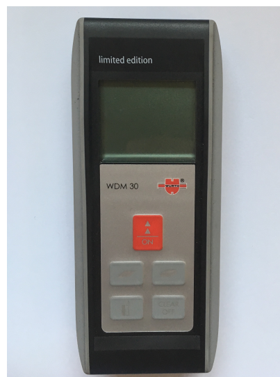
Fig. 4.5: Length measuring tool used to find the transformation between the reference frame and the chessboard.
