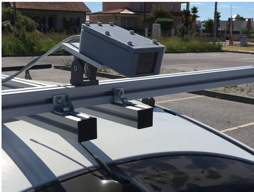
Fig. 3.5: Box that was created to protect the camera (Appendices B and C).
